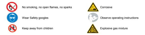
Labelling might vary due to application and dimension of the Battery. The manufacturer, respectively the importer of the batteries shall be responsible for placing the symbols (a minimum size is specified). In addition, consumer/user information on the significance of the symbols may be attached.
