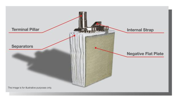
FIAMM SSLA RANGE USE AGM (ABSORBED GLASS MAT) TECHNOLOGY. THE ELECTROLYTE IS ABSORBED IN FIBERGLASS SEPARATORS WITH 99% INTERNAL GAS RECOMBINATION EFFICIENCY. BLOCS ARE GRANTS NON-SPILLABLE AND MAINTENANCE FREE THEREFORE REQUIRES NO TOPPING UP OF ELECTROLYTE DURING ITS WHOLE LIFE. LOW SELF-DISCHARGE ALLOWS 6 MONTHS SHELF LIFE.
