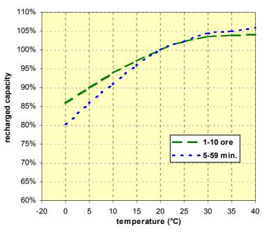
Fig. 4 Available capacity versus temperature
