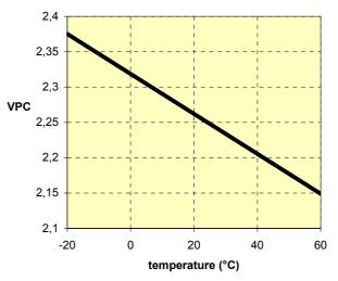
Fig. 5 Float Voltage vs. temperature
